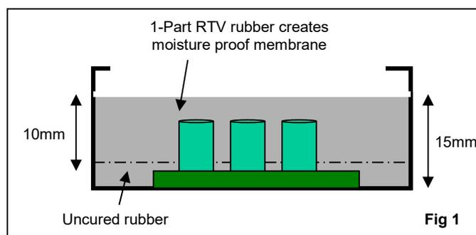
1-Part condensation cure (RTV) products should not be used where the depth of encapsulant is more than 10mm, see **Fig 1**, as it will cure to form a moisture proof membrane and prevent the cure in the bottom of the enclosure.
