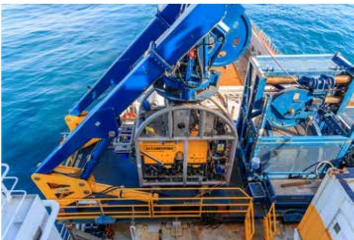
Deep-sea submersibles are connected to the surface operating ships via cables that carry power and communications. The single umbilical cables will contain several individual cables held within an outer sheath.
