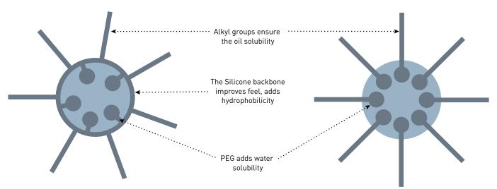
The Silicone emulsifier shown here, Cetyl PEG/PPG-10/1 Dimethicone, stabilizes the internal phase (water) within the continuous oil phase with a single emulsifying molecule. The advantage of silicone technology apart from imparting excellent feel is that the highly flexible backbone enables excellent emulsion stability across extreme temperature ranges.
